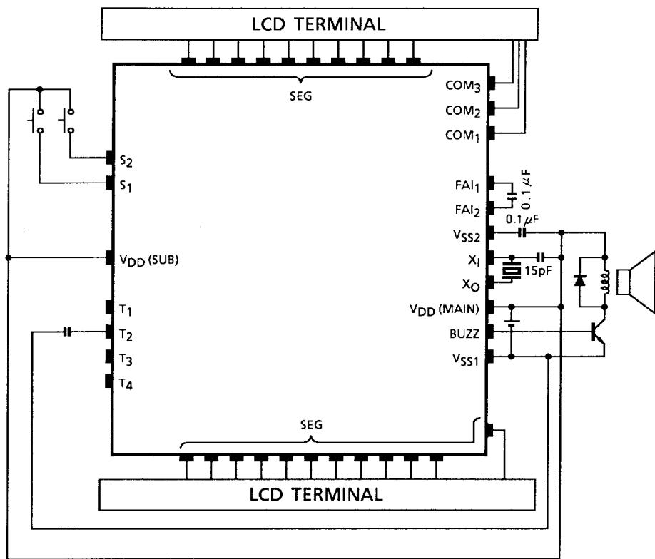
Note: Be sure to connect the V<sub>DD</sub> (MAIN).
